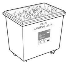
Big container, average weight 170 kg, tonnage 600 liter Width x height x depth (cm): 125,5 x 103,0 x 77,5
